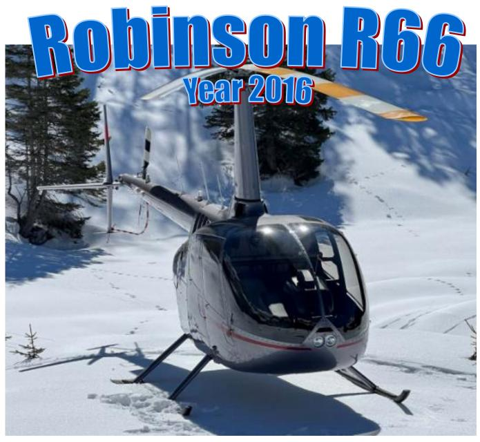
Manufacturer: Robinson Model: R66 Year: 2016 Airframe TT: 412 Hours Engine TT: 411 Hours Engine: Rolls Royce 250-C300/A1 Turbine cycles: 391
